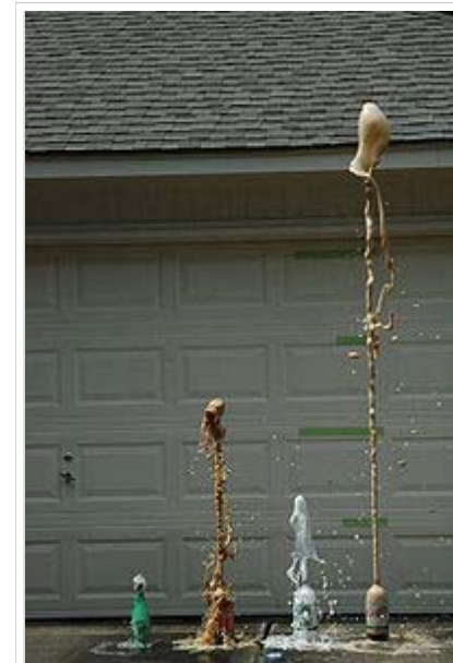
From left; Perrier carbonated water, Classic Coke, Sprite, and Diet Coke with 5 plain Mentos drops. Diet Coke presented a height about 2.5m.
